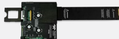
PE221UIA-X PCI Express 5.0 U.2/U.3 12 inch Interposer
